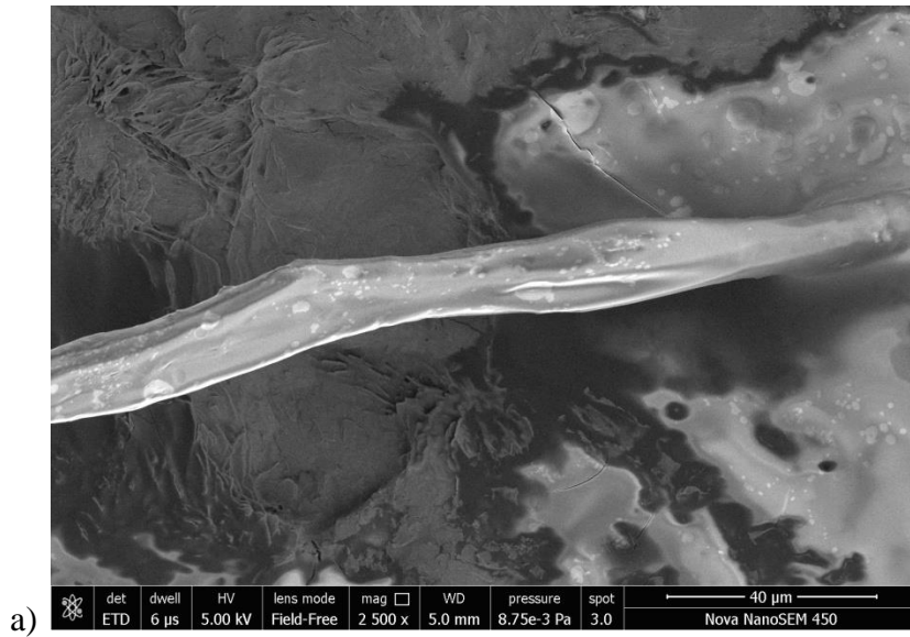
Figure 5: SEM image of the microplastic fiber sample taken at 2500X (a) and 1000X (b) magification respectively. Microplastic fiber is seen embedded over the filter paper membrane.
